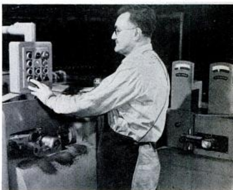
Scales at right weigh connecting rods and set cutters on machine to trim away precise amount of metal
